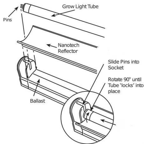
Replace the grow light tube by aligning the pins on either side and sliding the tube back into place.
